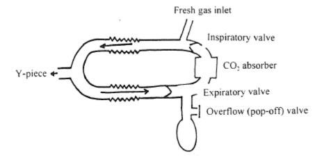
Which of the following components is misplaced in the circle system shown in the above illustration?
